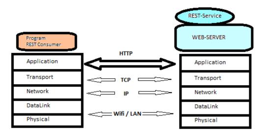
Figur A: Overall Architecture for a REST-Service
